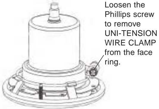
Spa light fixture with lens, gasket and face ring attached
